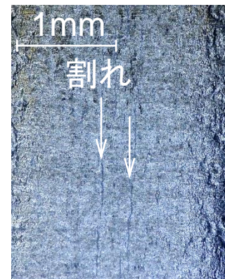
s = 6.0\text{ mm} 1500MPa鋼板, T = 400\text{ }^{\circ}\text{C}
