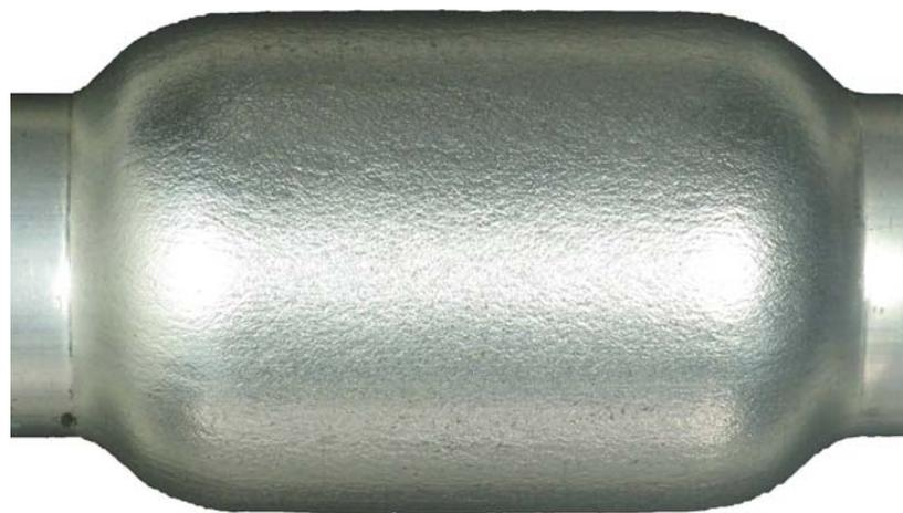
(c) SS400 ( $J=106\text{A}/\text{mm}^2$ ,  $t=4.0\text{s}$ )
