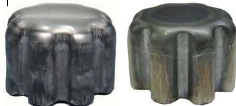
(a) 角部接触電極 T_c=640^{\circ}\text{C} , T=960^{\circ}\text{C} (b) 底部接触電極 T_c=630^{\circ}\text{C} , T=640^{\circ}\text{C}
