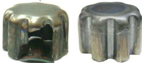
(a) 角部接触電極 T_2=310^{\circ}\text{C} , T_1=630^{\circ}\text{C} (b) 底部接触電極 T_2=630^{\circ}\text{C} , T_1=640^{\circ}\text{C}
